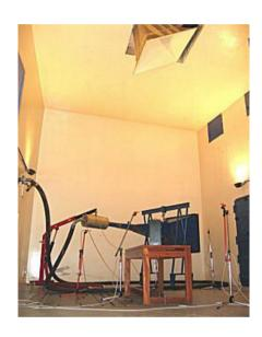
High intensity testing in the reverberation room can achieve overall sound pressure levels of 160 dB. Sound levels in excess of 170 dB can be achieved in a progressive wave tube in which panels are excited by grazing incidence sound.
