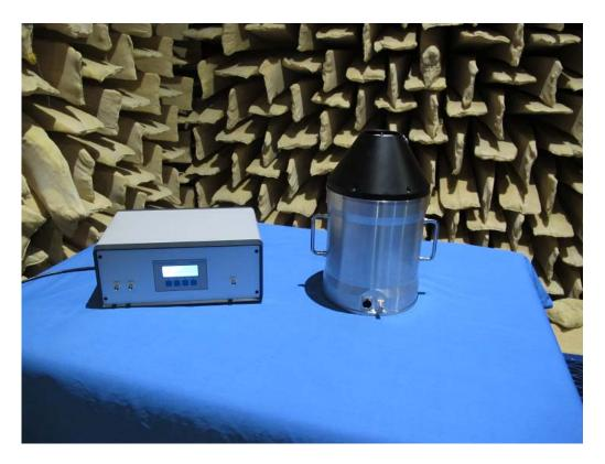
Figure 3. Low frequency source and the noise source power unit
