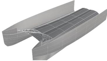
For monohulls, there was a need for a sheerline, keeline and chine line (for fast motor vessels), which are curves tracing along the points defining the station section curves of the hull. Within ISO 12215, for multihulls, in addition to these curves there is a need for –
