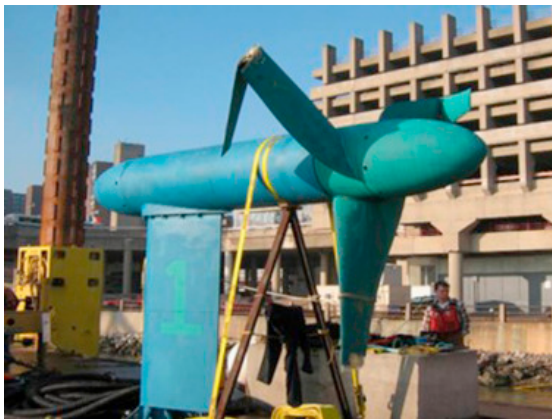
Fig. 4: Tidal turbine with broken turbine blades
