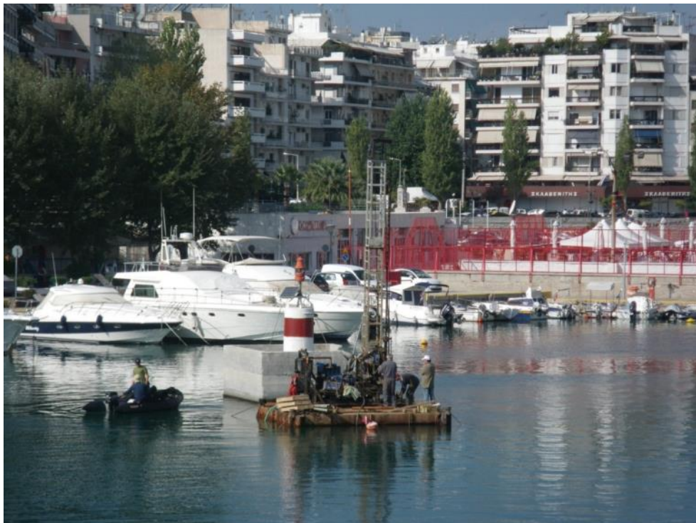
Offshore coring in the harbour basin of Zea, Piraeus, Greece (© CNRS - UMR 5133 / J-Ph Goiran)
