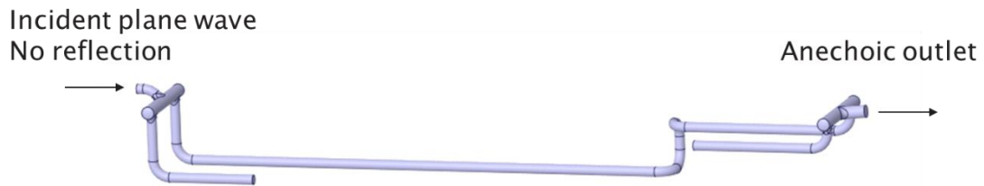
Figure 14: Duct layout with only single stream A operating and both upstream and downstream valves closed in line B.
