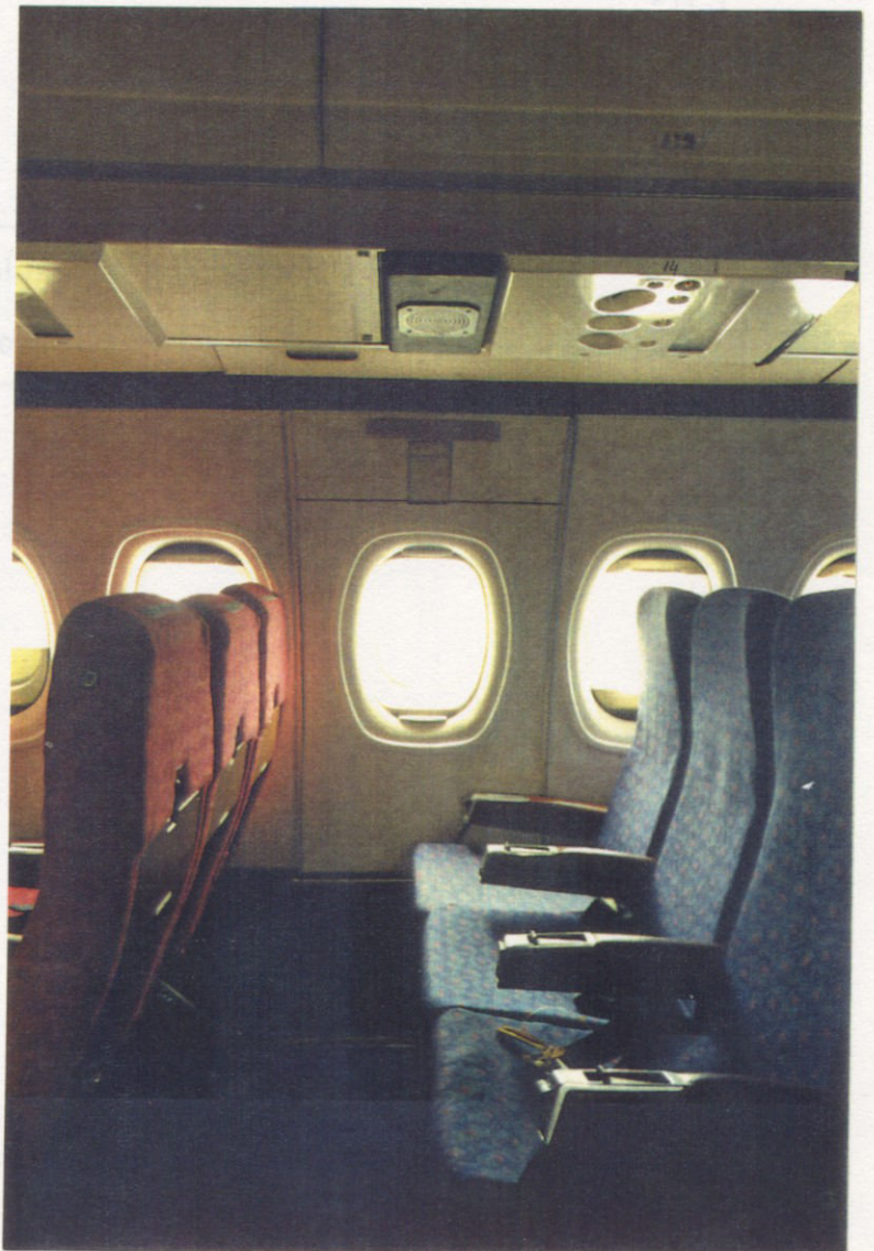
Figure 10 Audio attraction loudspeakers mounted in the Trident (a) In the bulkhead in front of the Type I exit (b) Above a Type III (overwing) exit
