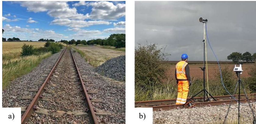
Fig. 2. a) View of test track b) The horn mounted above the test track
