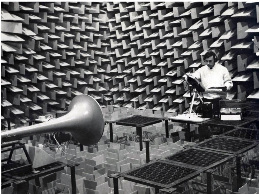
Figure 2. Sound level measurements in the original anechoic chamber, circa 1975
