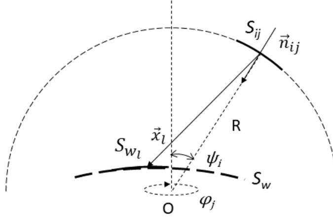
Figure 2: Diffuse sound field model using plane waves coming from various directions.
