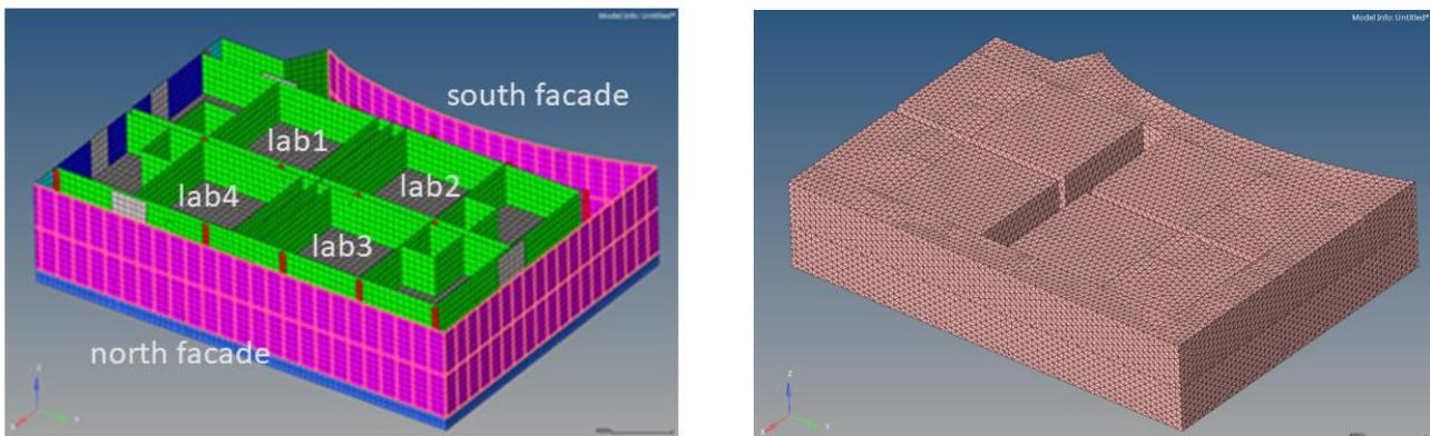
Figure 1: FE structural model of a science building showing all internal structural layout (excluding the roof), and modelled acoustic spaces shown in grey separately.
