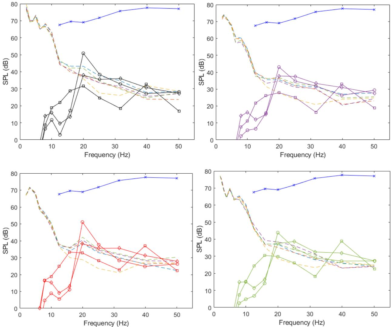
Figure 3: Comparison between the measured data (dashed lines) and the predicted data in the four labs; Lab 1 (black), Lab 2 (purple), Lab 3 (red) and Lab 4 (green), for the acoustic loading on the south facade (-o-), the north facade (-□-) or the roof (-◇-). The blue line is the aircraft SPL as measured outside the building.
