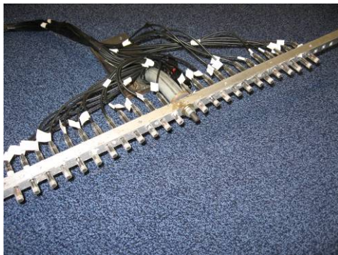
Figure 1 A simple linear microphone array
