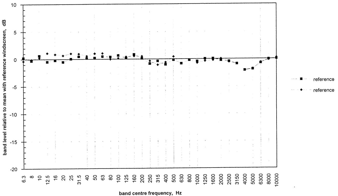
**Figure 37** One-third octave band SPL's relative to control windscreen (10 m/s)
