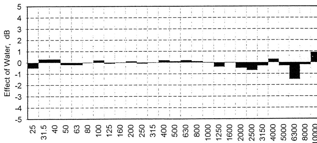
Figure 55 Effect of water absorption on acoustic insertion loss of windscreens
