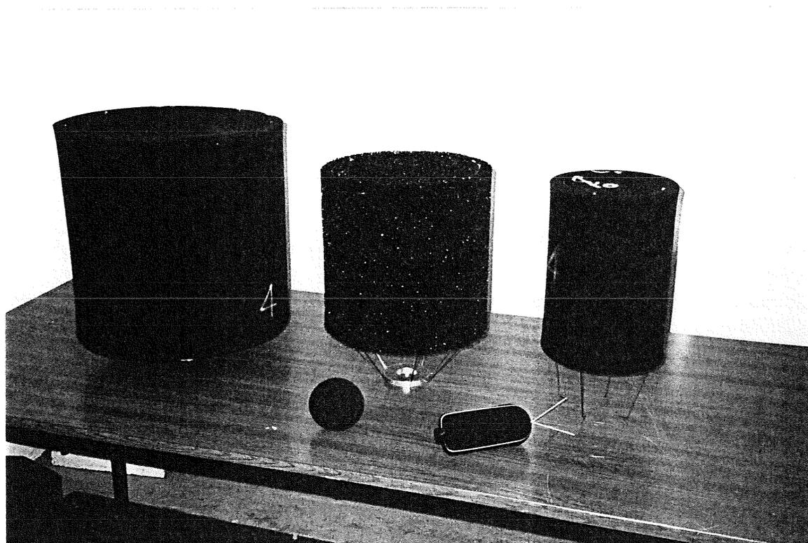
**Figure 8** 400/300/200 mm test windscreens with UA 0237/UA 0570 for comparison
