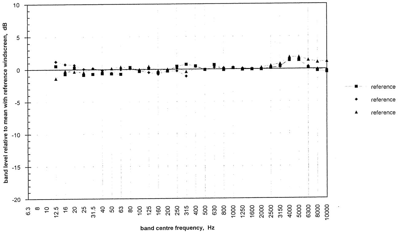
**Figure 36** One-third octave band SPL/s relative to control windscreen (10 m/s)
