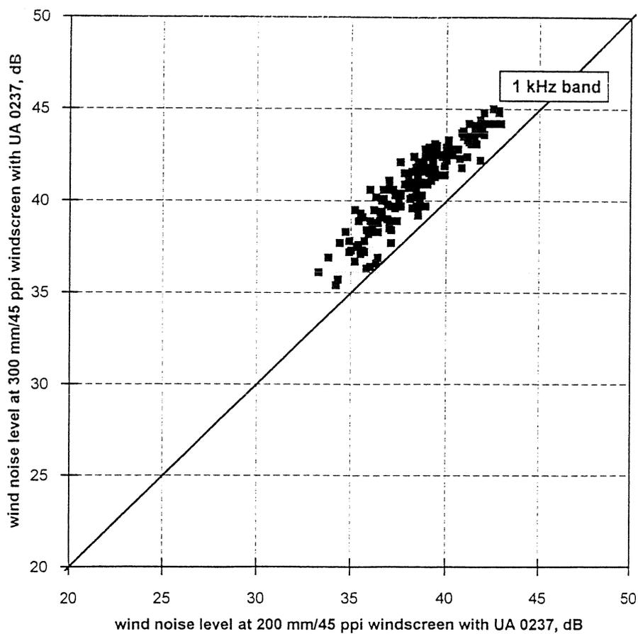
**Figure 52** SPL in 63 Hz and 1 kHz bands plotted for 300 mm/45 ppi and 200 mm/45 ppi windscreens
