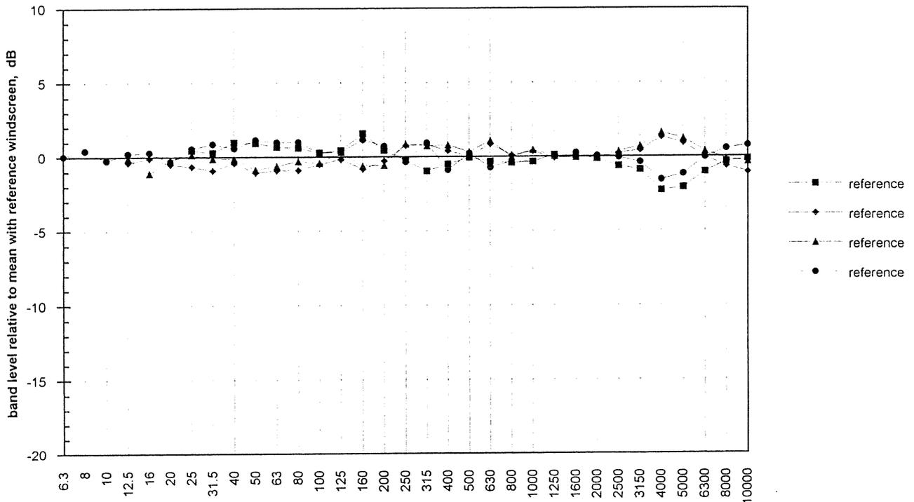
**Figure 34 One-third octave band SPL/s relative to control windscreen (10 m/s)
