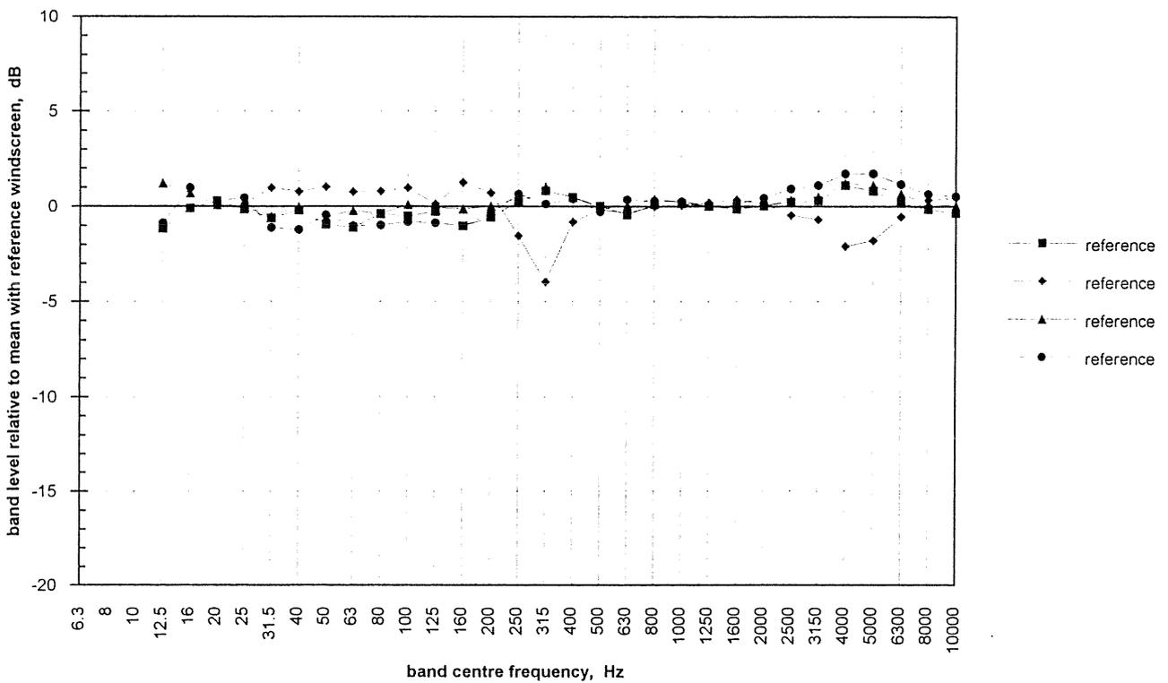
**Figure 35** One-third octave band SPL/s relative to control windscreen (10 m/s)
