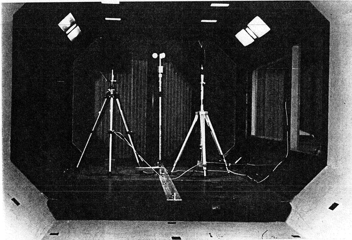
**Figure 19** Installation of windscreens and anemometer in 7' x 5' wind tunnel
