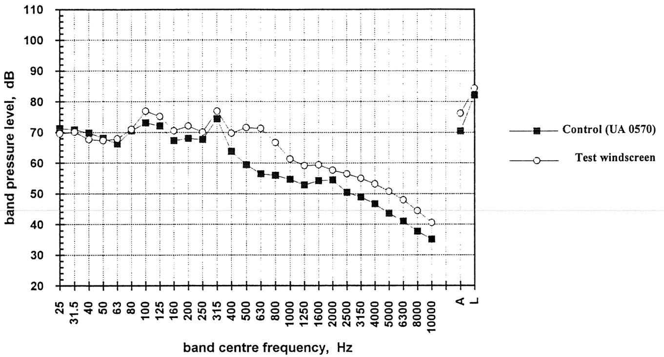
Figure 24 10 ppi hollow windscreen -v- UA 0570 - smooth flow 10 m/s
