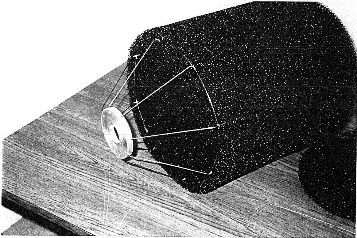
**Figure 5**      **Mounting plate at base of windscreen**
