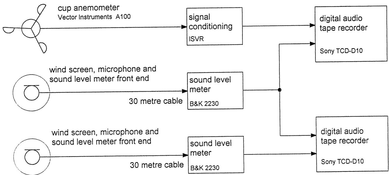
**Figure 18 Measurement system for wind tunnel and outdoor measurements - schematic**
