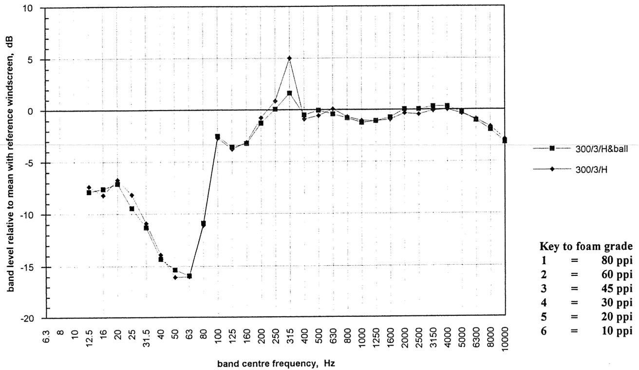
**Figure 38** One-third octave band SPL/s relative to control windscreen (10 m/s)
