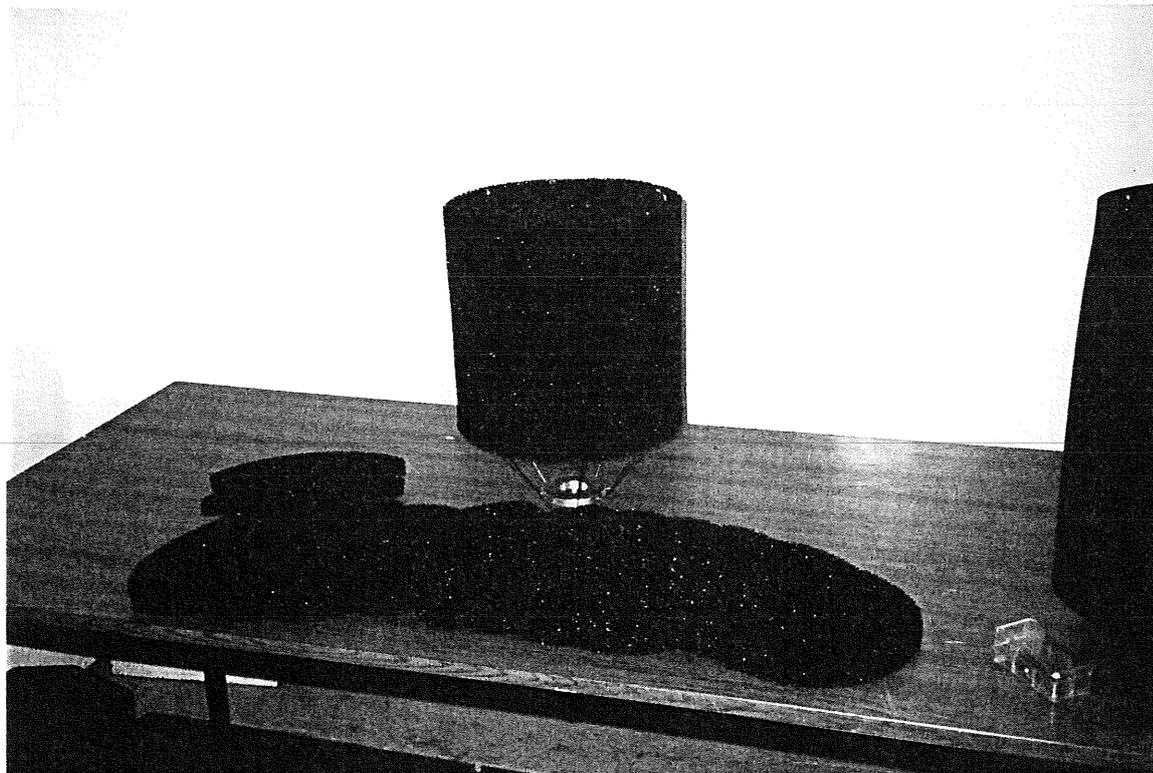
**Figure 7** Construction of solid windscreen using stacked discs in outer sleeves
