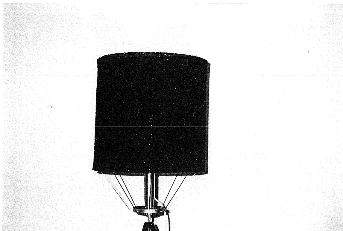
**Figure 4** Installation of outer sleeve (10 ppi) on windscreen
