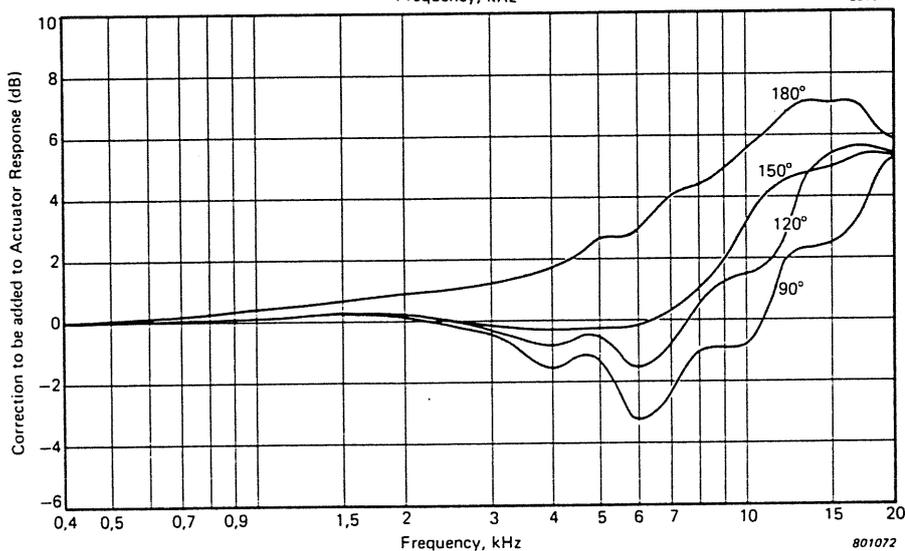
Fig. 9.7. Free-field correction curves for half-inch microphone Type 4133/49 fitted with Rain Cover UA 0393 and Dehumidifier UA 0308 mounted inside Windscreen UA 0570
