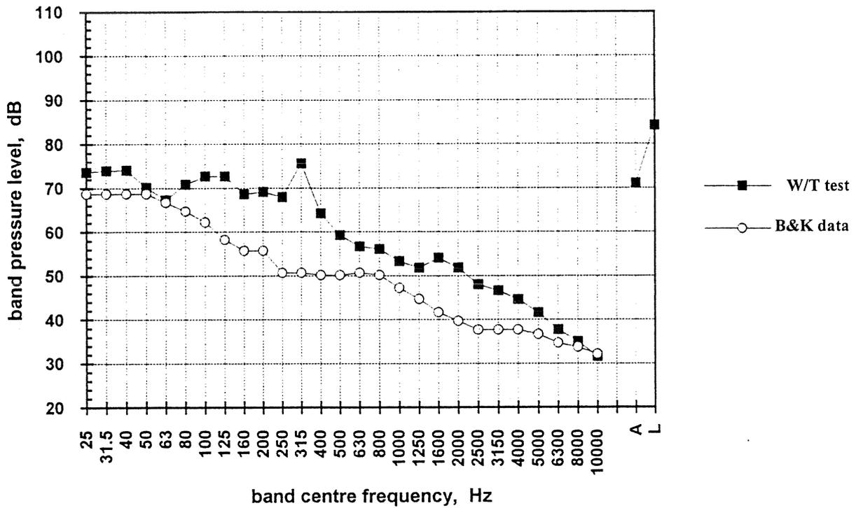
Figure 21 UA 0570 in wind tunnel (without 0393) -v- B&K data for wind noise
