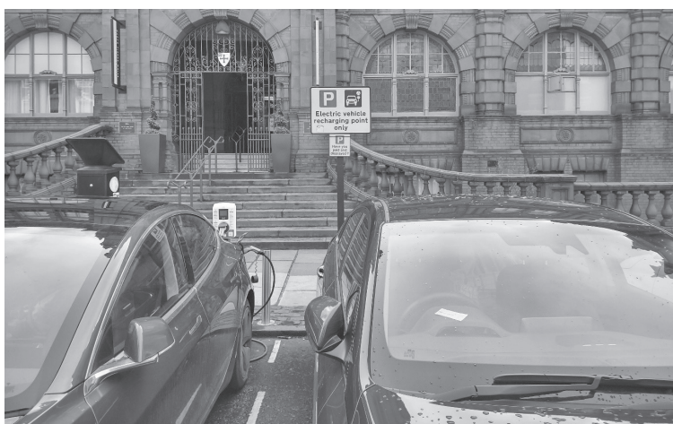
Figure 2: An on-street electrical vehicle fast charger in Durham city centre. This is again illustrative of the lack of space for wheelchair users driving EVs who want to make use of these charge points.
