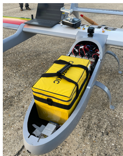
Figure 2. The Mugin V5 Pro hybrid drone being loaded with chemotherapy treatments
