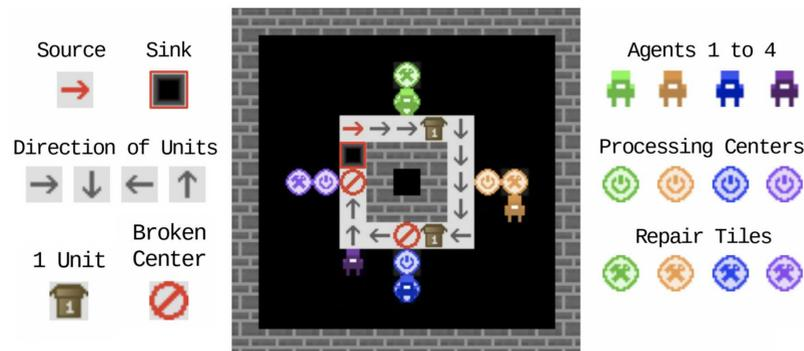
The environment is a 2D gridworld with an underlying graph structure in which agents must process units while maintaining their own individual processing centers with the help of other agents.
