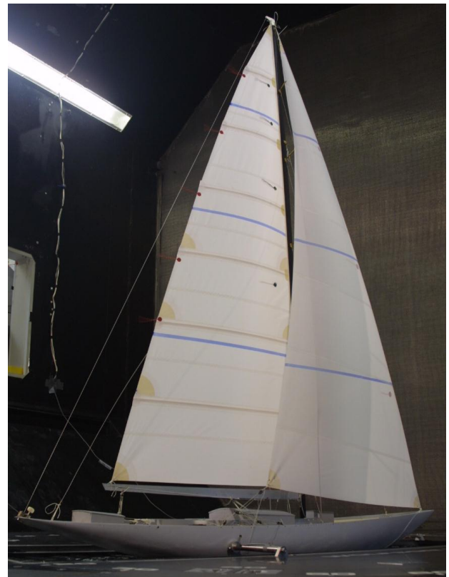
Figure 6 Model used for maximum heeling moment tests.
