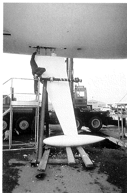
P. 15: Mike Plant's Coyote – a recent victim of bulb detachment. Top: Martela OF after keel failure, Whitbread 89/90. Above: Martela's keel already straining after leg 1. Right: Fleury Michon – three days into the Vendée Globe
