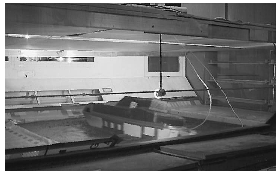
Figure 8 Conventional catamaran during gust test
