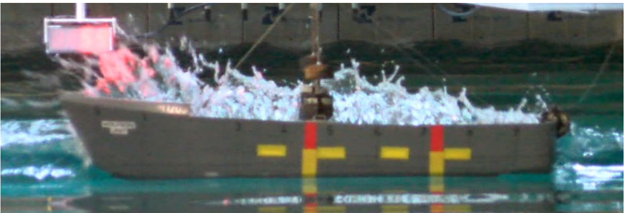
Figure 19 Open boat, loading condition 4.2, run 59: wave height 1.20 metres, wave period 2.8 seconds
