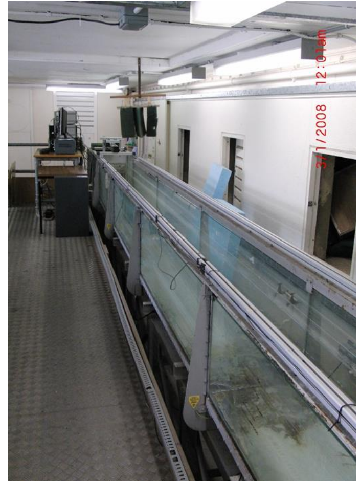
Above: 0.4 m wide wave tank Above left: 12 m long flume Below left: General purpose flume (foreground), 15 m wave tank (background)
