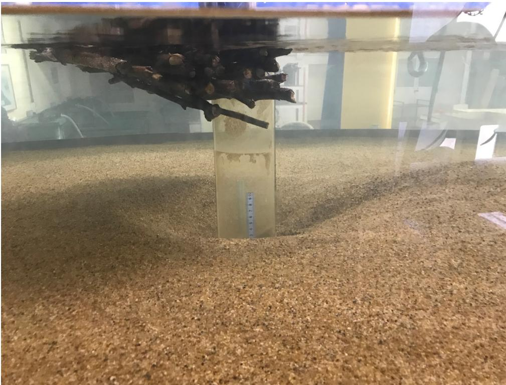
**Figure 6.** Example of woody debris models used during the experiments conducted at the University of Southampton and its impact on scour.
