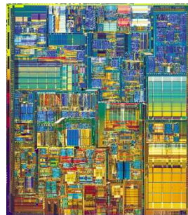
Intel Pentium-4 (2000) 42,000,000 transistors 0.18 \mu m process
