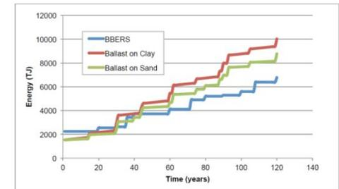
Figure 6.1: LCA of different forms of railway track with minimum steel EE
