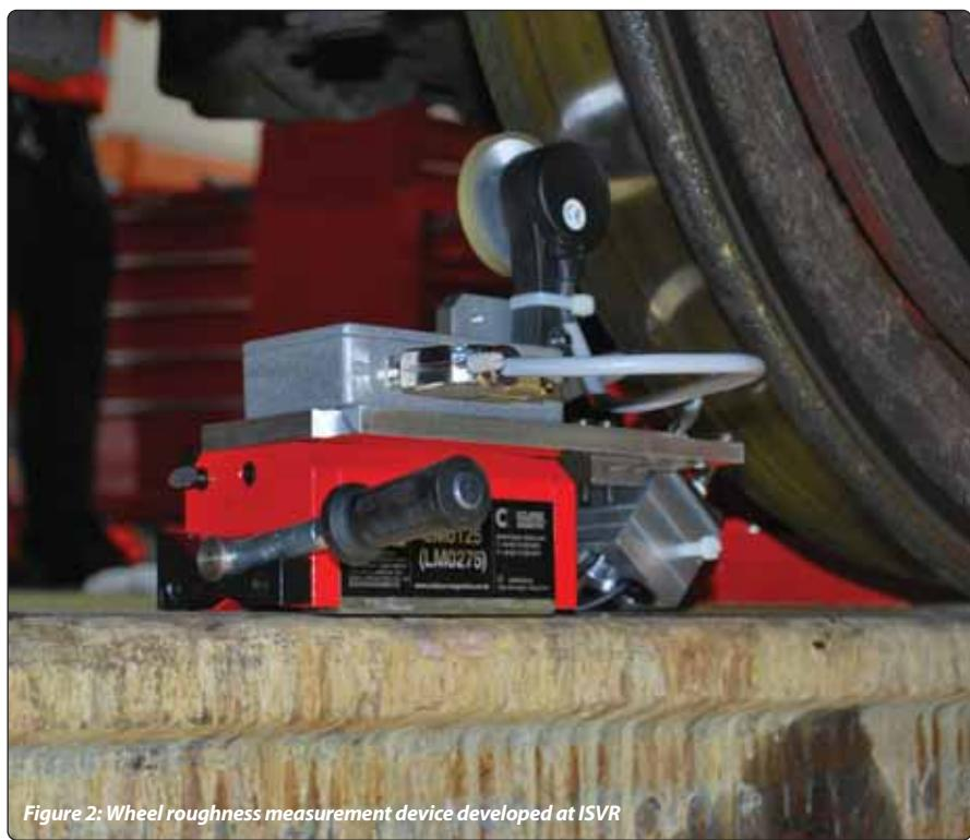
**Figure 2:** Wheel roughness measurement device developed at ISVR
