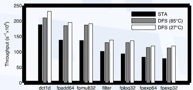
Figure 4. Throughput comparison with static voltage constrained DVFS
