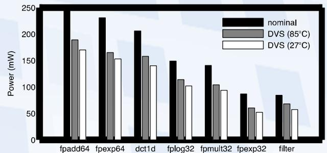
Figure 3. Power comparison with static frequency constrained DVFS
