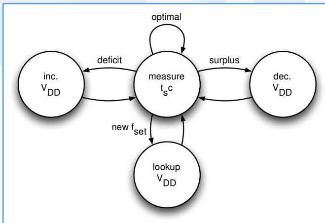
Figure 2. Diagram of the interactive frequency constrained DVFS controller
