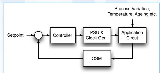
Figure 1. Block diagram of the DVFS controller
