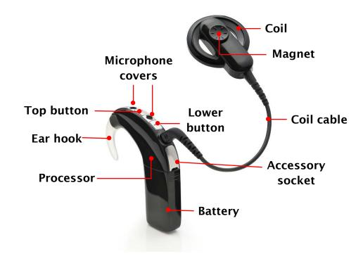
Switch 'on' by connecting the battery, 'off' by disconnecting the battery
