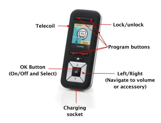
Switch your remote control 'on' or 'off' by pressing and holding the Ok button
