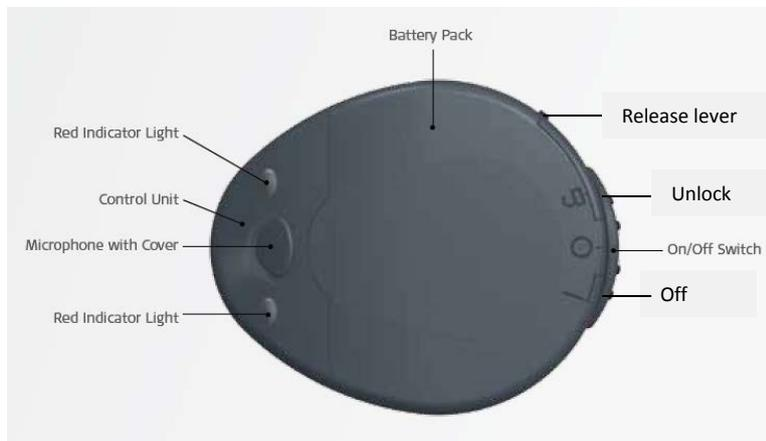
To open the battery pack, hold down the release lever and slide the switch to the unlock position. Then lift the battery pack up. This will enable you to insert the batteries – make sure that the positive side (+) faces upwards, towards the outside. Slide the battery pack into the control unit, push it down and then slide the switch to the locked position (O). To turn the processor on, slide the switch across to the I position.
